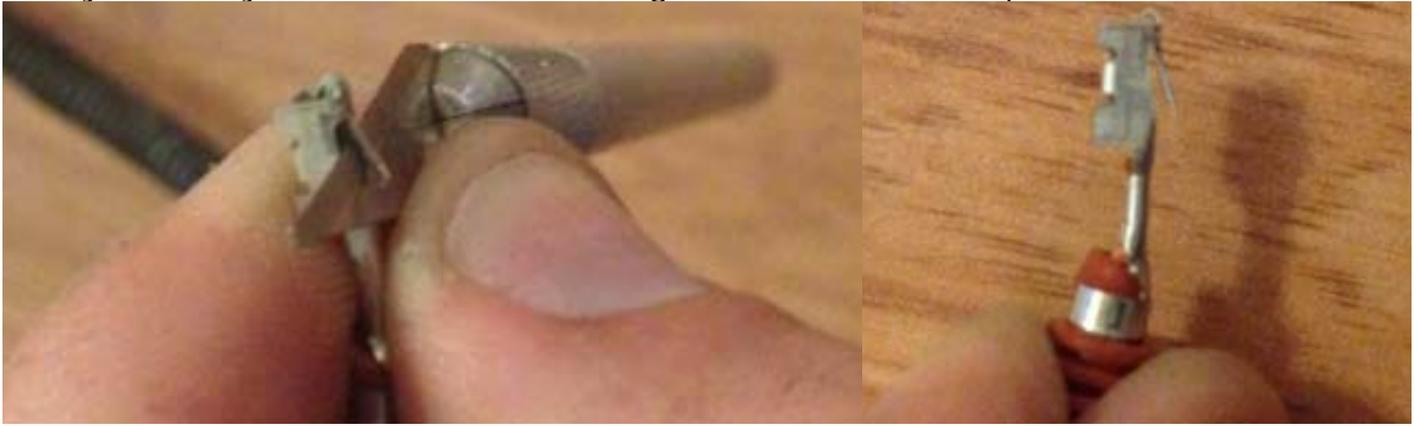
Now, slide the old pin into the new connector. Make sure that you rotate the pin, so that the locking tab will slide into the groove seen on the front of the connector housing. Also, put the colors back into the location you removed them from. Refer to the diagram above for which color goes where. Re-install the pin-retainer onto the back of the connector shell.
